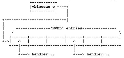
The OS initially allocates 8 VBI slots. The first slot is reserved for GEM's VBI code. To add another deferred handler, place a pointer in a free (NULL) slot. If there are no more free slots, then allocate a larger VBI array, copy the current vectors to the new array (clearing any new, unused entries), and update vblgueue and nvbls.
